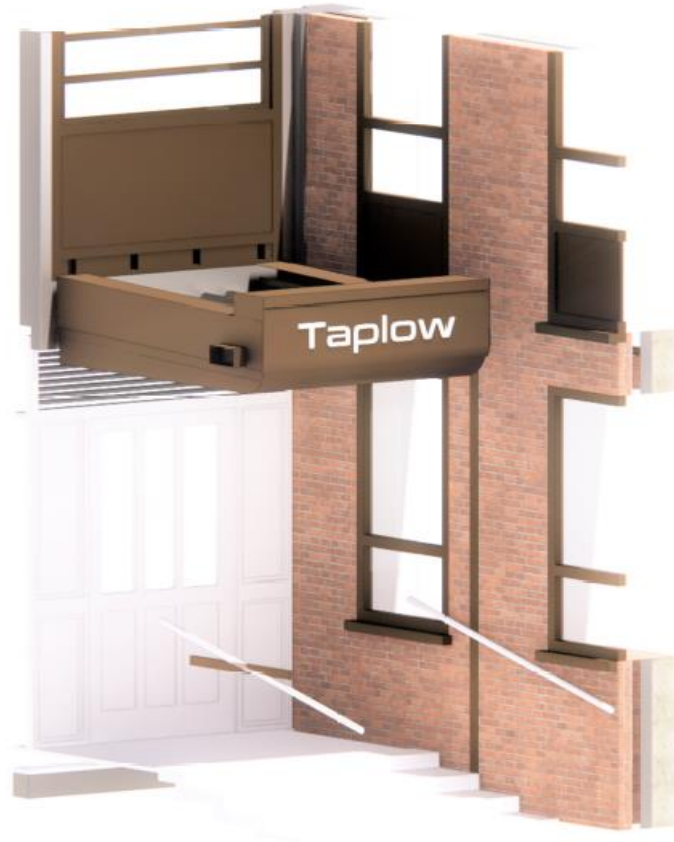
3D VISUAL - TYPICAL CANOPY ARRANGEMENT
